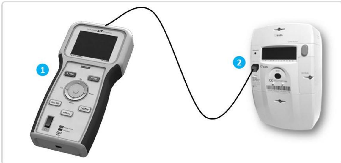
Figure 6: Connecting to a smart meter
